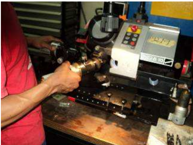
Figure 16: Carlo exercises and grinds until the drill "ok" is. We tested whether he drilled well and if the diameter is correct, it is good. Now people are trained by the "Machining". If they do not have enough work, then man is there, the drill can regrinding.
