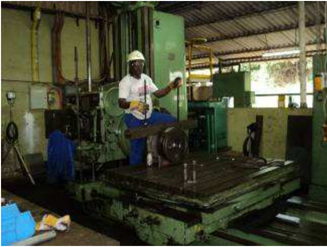
Figure 29: This old Union has built in 1950. This machine is taken once a year were examined in detail, so that spare parts can be ordered. If necessary, redesign to newer parts.
