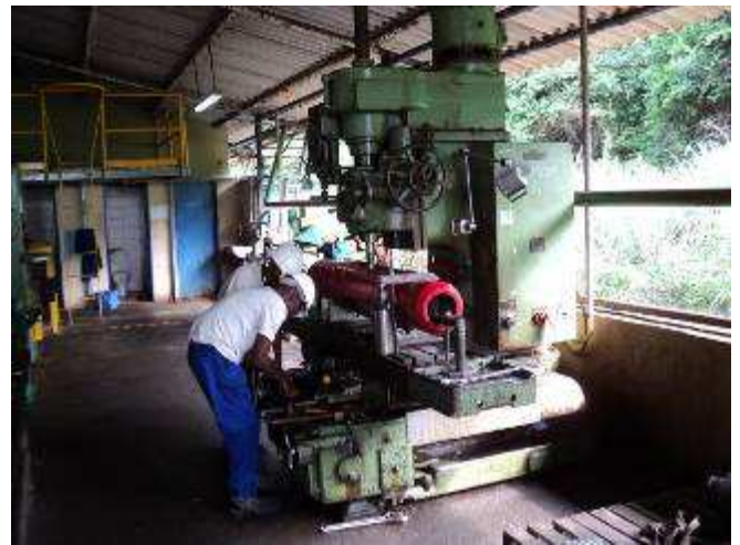
Figure 17: There was a message that no longer goes to the Hermann milling the feed. The feed gear box had to be opened.
