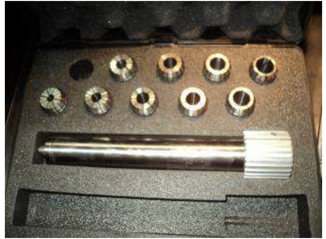
Figure 13: Here clamp the various grippers to drill. This machine can be used up to 20 mm and for cylindrical drill shafts.
