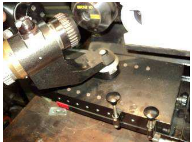
Figure 14. Here, the drill is clamped, so that it is horizontal on the line next to the optic at an angle and the 180 degree lock is locked. So both sides with 10 degrees can be geschlossen evenly.
