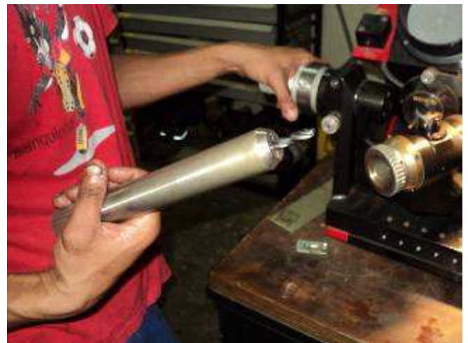
Figure 11: The drill bit is clamped in a chuck, then one can grind with 2 angle. identical first to 10 degrees both sides so that the center is true, then at 30 degrees.
