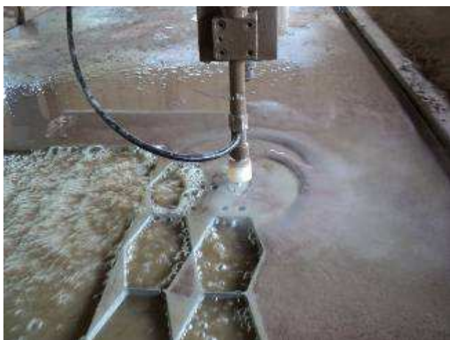
Figure 4: Within minutes are sol cut any contours. Deburring is not necessary, the edges are rounded.
