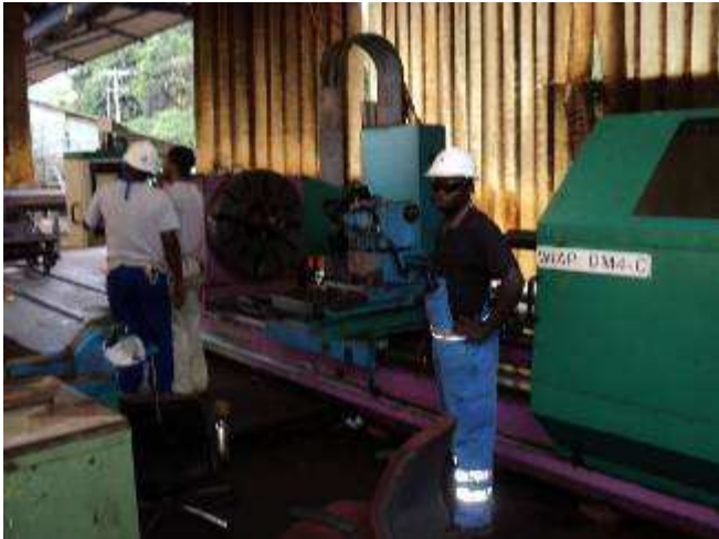
Figure 26: This Gurutspe WIAP DM4 C has the same machine bed and compound slide as the Gornati, but just the headstock of a Spanish machine
