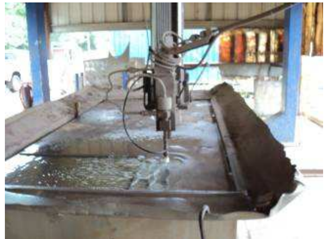
Figure 2: This machine can ca 0.1 mm accuracy, cut parts. Only water is used for plastics, rubber. Add to this mix abrasive, ie something like sand and water, stainless steel can be cut as with a knife.
