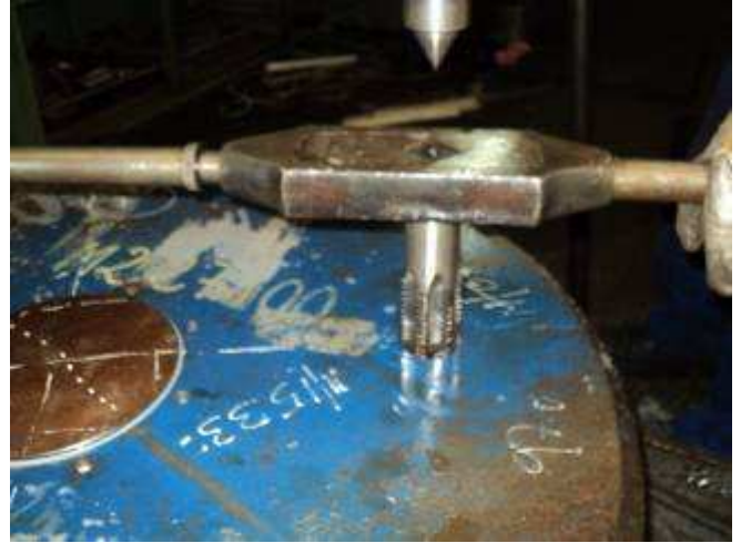
Figure 31: Every time the strong men turn the wrench is guided from above the tap. In order to reschedule the wrench, the hydraulic clamping of the machine must be released and re follow up. Obviously these people who work here, decades of experience; this will be noticed immediately. Actually watching a pleasure. It is also apparent that much knowledge come from Swiss apprenticeships and other countries. What these people know today is only to be admired.
