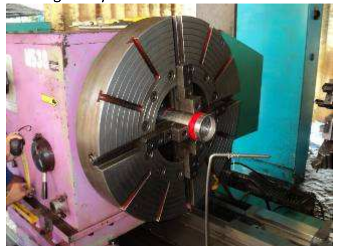
Figure 25: This is the brother of Gornati lathe Gurutspe. Only the headstock is from the old conventional machine. The bed and the carriage with revolver and CNC control is
