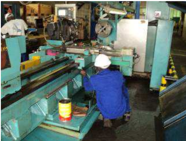
Figure 15: It is prepared everything to lift the sled. Under handles away. Ballscrew away etc
