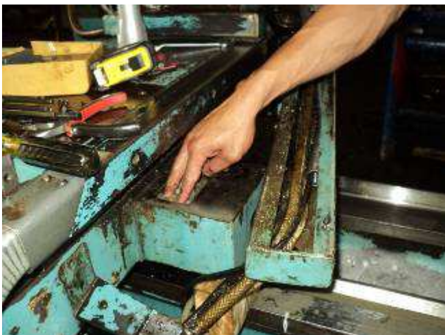
Figure 29: This was the old Oelstelle from the old conventional system. Safe 2 liters of oil was in it and smeared the old time itself. But with the construction of a CNC machine these old grease variants were no longer used. It was attached to the central lubrication system. This are now these old oil container full of old emulsion.
