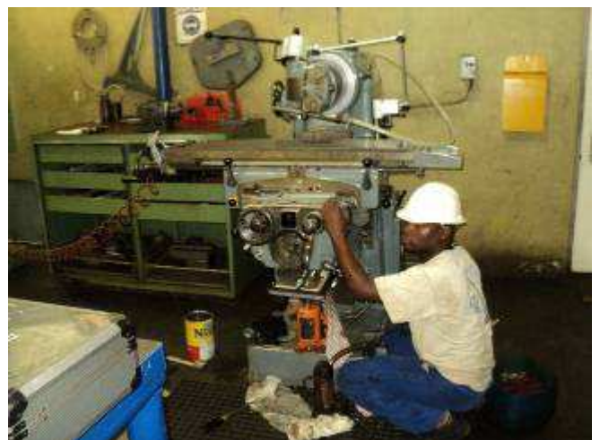
Figure 8. After Niles lathe comes the Schäublin milling machine turn. There is a clear-year plan, when, what equipment needs to be serviced. All machines are serviced.
