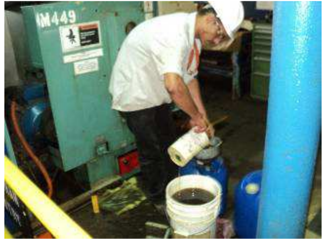
16: But the oil is replaced. The tank is cleaned inside. Often there are problems with the "bosses" of the "Machining" department to get the equipment for maintenance. Recently we had to them, say how many times: whether they know why almost no planes fall down today? Only because of the preventive maintenance. It was then said that one purpose is to force that they can release the machines!
