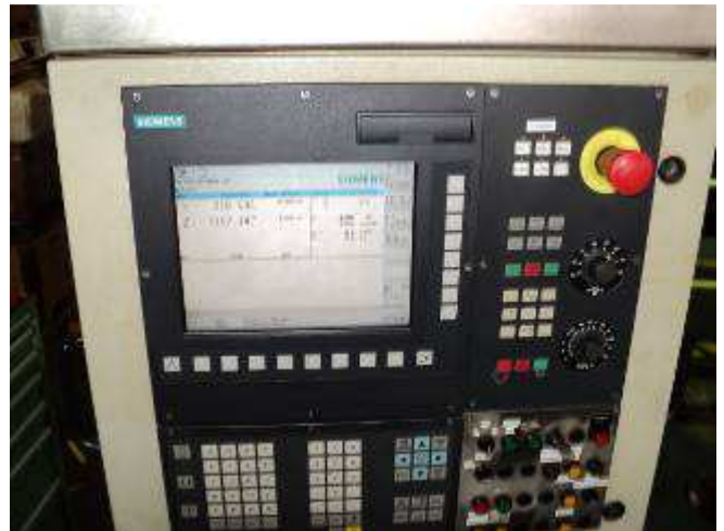
Figure 17: This is the CNC control, we grew in the year of 2006. The previous Sinumerik 810T is long gone in use.
