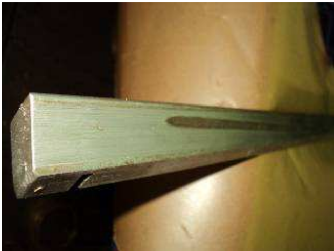
Figure 5: take out wedges and clean everything, ready to scrape at the next service.
