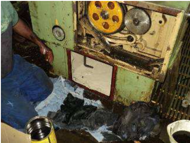
Figure 4: oil change at all next machine. And clean the oil tank inside.
