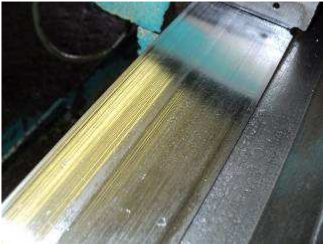
Figure 14: It has running tracks. However, since this affects in contrast to a slant bed machine, only the top level, it has no major impact on the accuracy.
