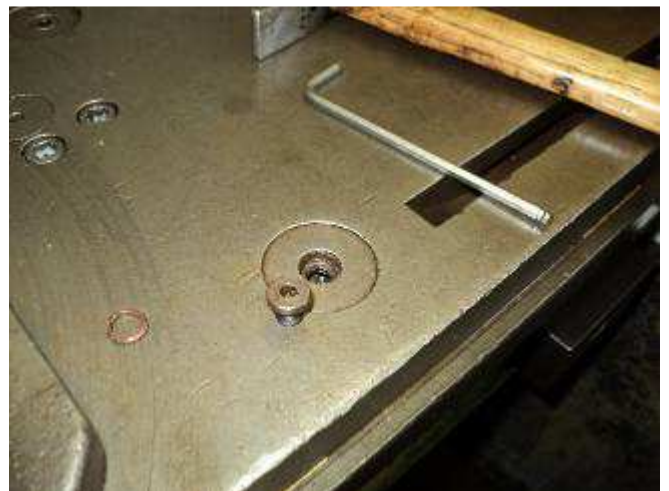
Figure 7: The fact that lubricating points are under the screw from the X slide, is marked in the future with a red color.
