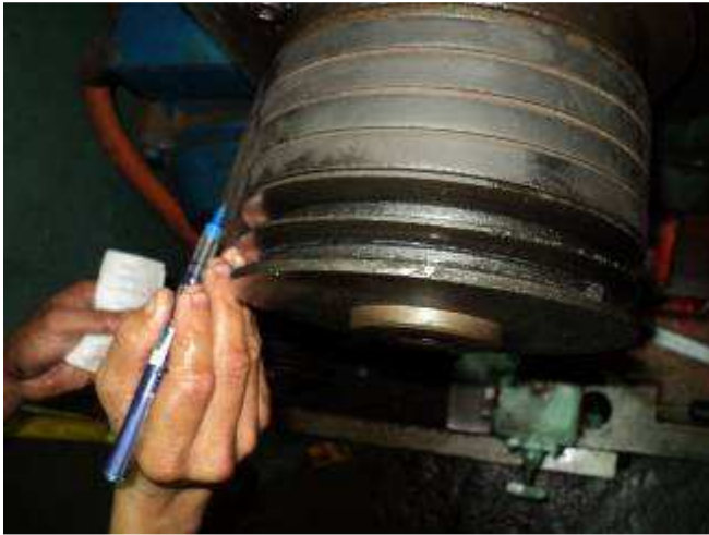
Bild18: The V-belt of the spindle motor also look not good. We have now expanded our maintenance list so all machines covers all belt with storage location that is bearing number. What is missing is ordered. The yes only cost a few dollars. But if it's not here, it costs a lot when you have to let it send by DHL. Our young people will keep but now encouraged so that they have at least once from all major machines, a set of belts in stock.
