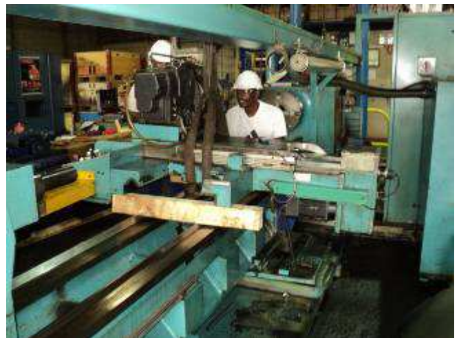
21: Now the carriage sits on timber and is ready to examine why the guides have these running tracks.
