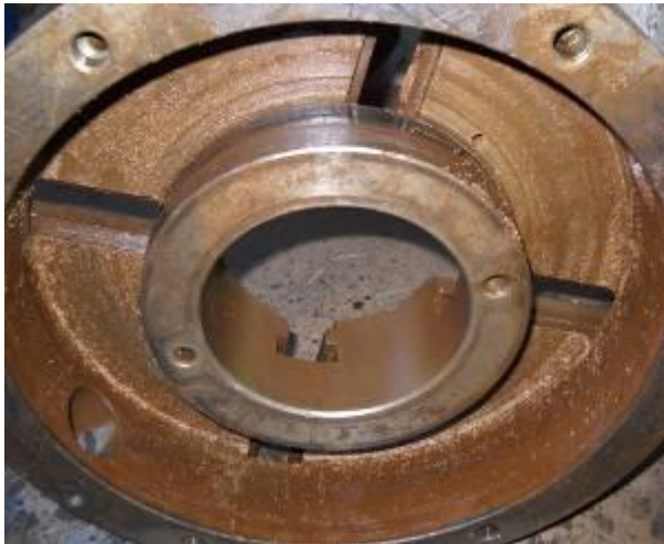
Figure 6: disassembled and cleaned inside lining
