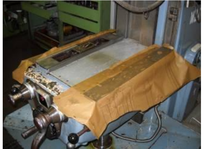
Figure 6: During repair work should always everything will immediately covered with oil paper
