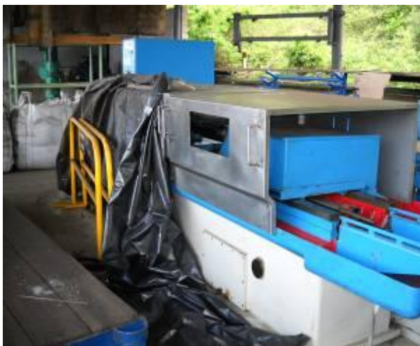
Figure 7: This Tiefbormaschine is normally covered if they do not have to work. However, when the wind blows away the cover and it remains open one week, the rust eats on the guides.
