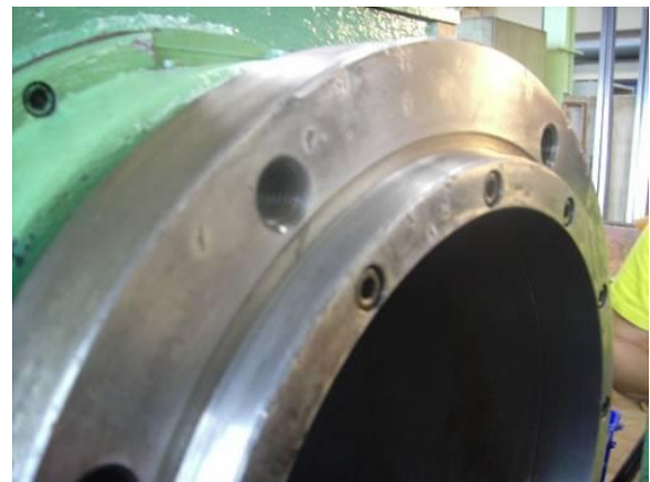
Figure 2: spanning hundreds of impressions from the dirt at the food. Only with a whetstone can correct these damaged surfaces again. That is, eliminate the increases so that the concentricity of the chuck is good again. But that stretched across the dirt that is not good!
