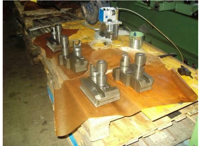
Figure 4: Here the cleaned clamping jaws. It takes about 4 hours of work to make everything clean.
