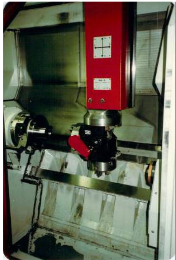
The swivel hook with self-locking gripper when power failure, that the workpiece will not drop it. The gripper can be 0 and 90° plus 180° rotation. WN_1220_40
