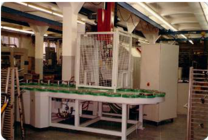
A self-developed raw and finished part storage. WN_1220_20
