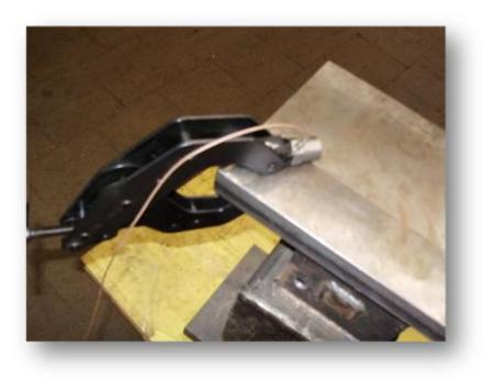
The measuring probe as it is mounted on the workpiece. Always use caution; the cable is very sensitive and should also not be "kinked".
