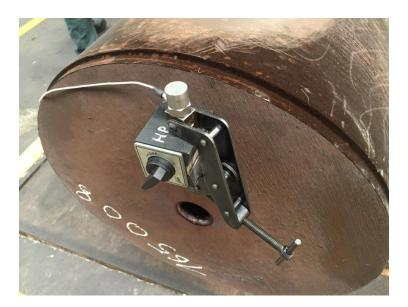
Photo: The measuring probe as attached to the workpiece With solenoid Please Achrsichtung of excitement .When note 2 D vibration is always an axis untouched ie the probe is to check the axial direction, which is touched.
