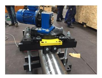
14. 4.22 prisms set for round parts up to 800mm
