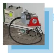
The equipment for dimensional stabilization by vibrations is a portable one and can be used for parts having any size, shape or weight resulted after welding or casting and for other structures. The small parts can be treated by fixing them on a shaker.
