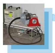
The vibratory stress relief equipment with microcontroller, in its variant with maximal fitting out, comprises the following elements:
