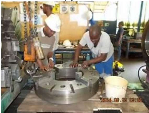
Figure 29) The feed was dismantled, cleaned and the injuries deducted. The defective spindle repaired temporarily until a new spindles there is.
