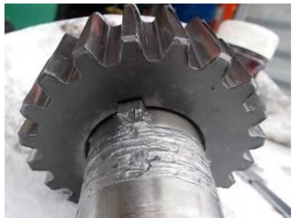
Figure 70) The large gear: The shaft has sheared the wedges.
