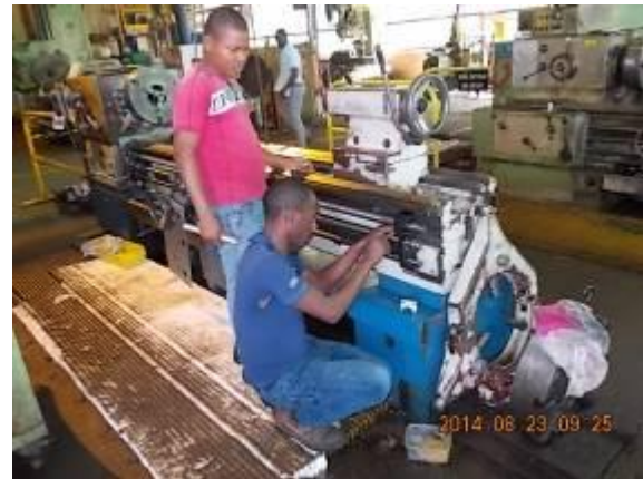
Figure 45) The re-assembly in the process. Yoba and Bambi. Kevin brings new belt and a new thrust from Switzerland.
