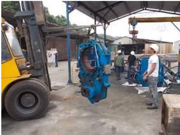
Figure 61) The inner member is removed to disassemble.
