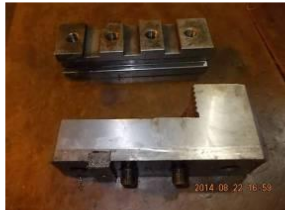
Figure 26) The shoe has dumped because it was too far out.
