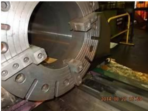
Figure 24) Here, the operators have with the WIAP Gornati these very good jaws of 4 years old faceplate eager to ensure that the threads are broken out so far at the back spindles. Just because they were too lazy to push the upper jaw forward. It is clear that the
