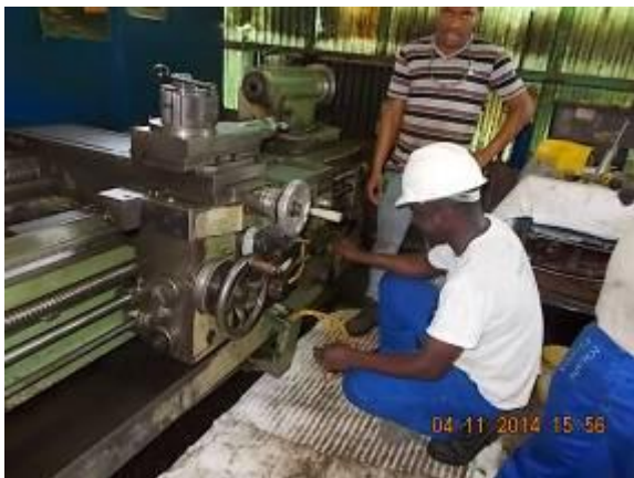
Figure 57) After approximately 4 working days of the carriages was refitted.
