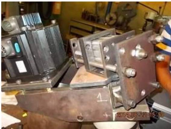
Figure 8) This is now the belt brake with the 63-cylinder. He presses with 6 bar, 164 kg.
