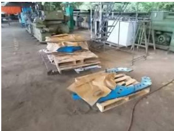
Picture 71b) Until the spare parts in Angola, the demonitierte goods must be well protected. Lightly oil / grease and cover with oil paper.
