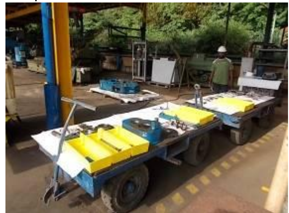
Figure 65) order and clean dismantling helps that no assembly mistakes.
