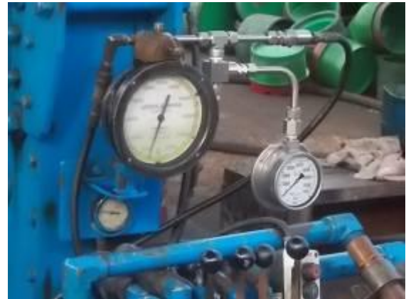
72) An extended manometer solution facilitates working on the machine.
