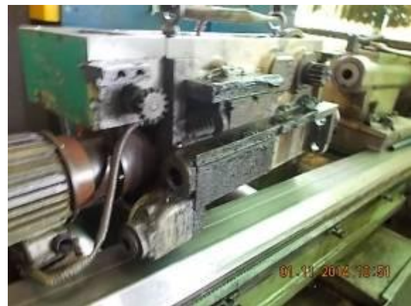
Figure 49) at the Niles lathe has now once demolished 3 a pen. Once pushed off the Axiallagerbock and torn.
