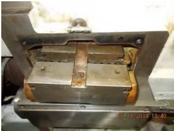
Figure 56) This split nut jammed and did not go into the self. She stopped occasionally hanging in the trapezoidal screw and blocked.
