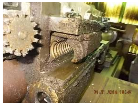
Figure 49) at the Niles lathe has now once demolished 3 a pen. Once pushed off the Axiallagerbock and torn.
