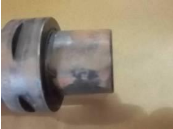
Figure 23) This is a Sandvik Capto tool holder 63. Which costs a few dollars. rusted located outdoors and, No rust protection.
