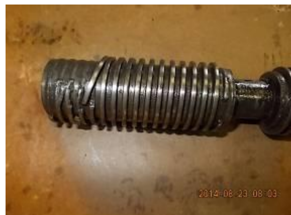
Figure 27) on the spindle pressed off the thread.
