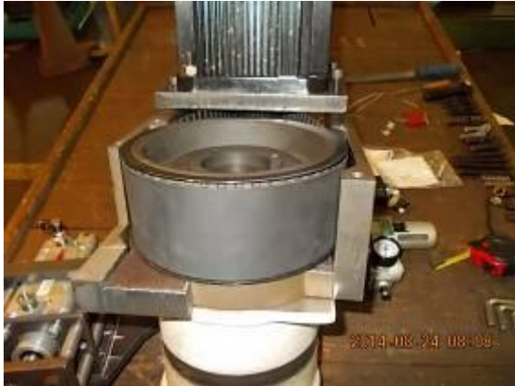
Figure 7) on the motor extension we made the motor with a rotary flange. So that we can turn the engine in any surrounding location.
