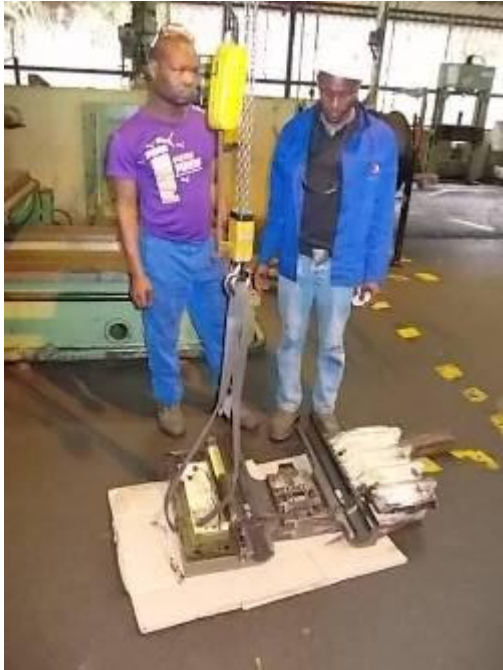
Figure 38) and Antonio Yoba recover after removal of the longitudinal slide.
