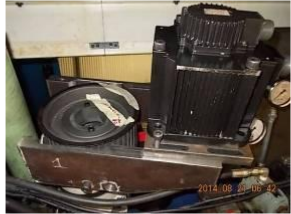
Figure 5) The X motor 1/3 stocky with 3 kW. The old engine had 7 kW and was 1: 1. However, only 10 M Rapid with a 10-er ball screw.
