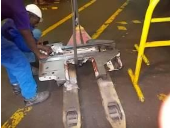
Figure 43) The cross-slide is prepared again for the assembly after a thorough cleaning.
