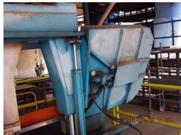
Figure 46) Here, a band saw Knuth from Turkey. It stands about five years here. The color is probably a new, water-soluble paint. It drops. we need new and well paint on occasion this machine.
