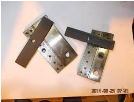
Figure 44) Again, due to the V guide, the lower handle that is not so old machine TUR is so loaded that it has the sliding coatings, demolished by the transverse forces and then press the intense upward. We had to re-roughen the bonding surface so that it has cavities for the adhesive. Then re-bonding. with brass for countersunk screws against the re-tearing of the sliding coatings.
