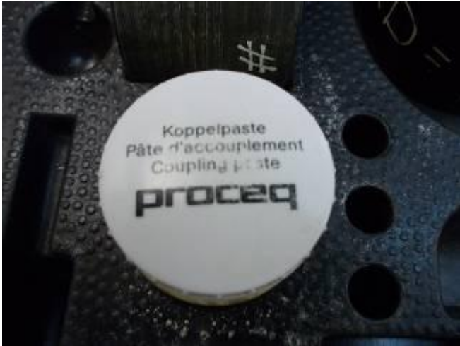
Figure 6: This coupling compound is packing in the meter. This is required when the workpiece is easy.
