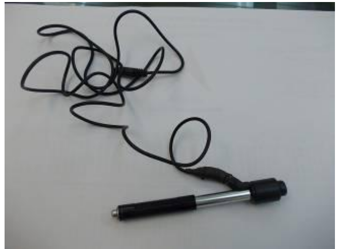
Figure 9: Impact Device D. put away caution when devices. packaging the lateral plug down.
