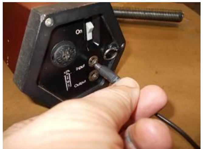
Figure 10: The impact device is connected here on connector Input
