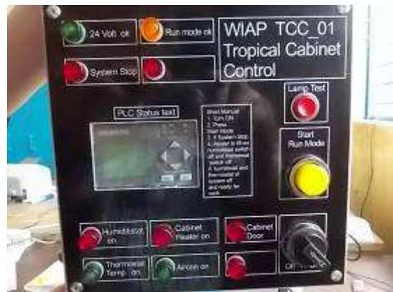
Photo 4: We started 20 Tropical Cabinet Controller for Angola. There, the condensation always destroys the electronics.
