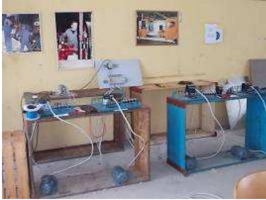
Photo 16: Protecting square test with 4 Motors - counterclockwise and clockwise rotation.
