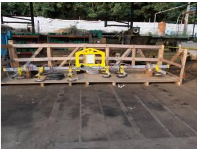
P58: Vacum Heber. Who was appointed for the waterjet machine, because there's a lot of stainless material.
