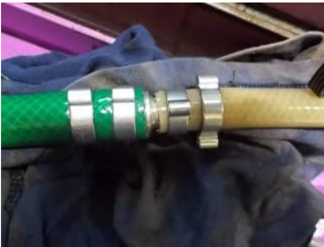
P23: A new clutch rotated and attached double hose clamps
