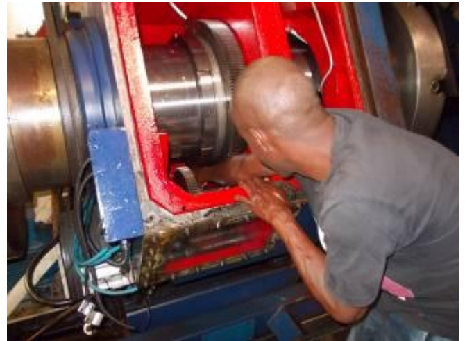
P9: Below, under the oil, is a flow filter. Only accessible with a very long arm.
