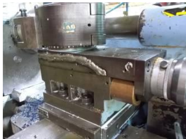
P40: At the Storebro 260 GS the top slide is broken. Make a new one. Organize cast iron.
