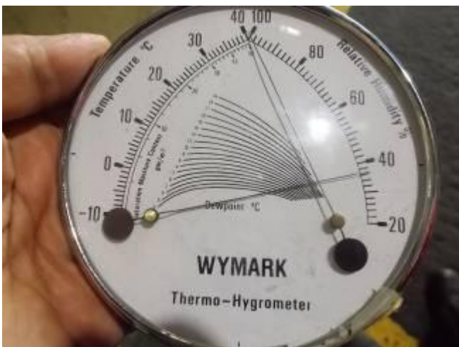
P43: For the Weisser CNC lathe we needed the thermometer, which we had forgotten in the closet of Gurutzpe. Just 40 degrees Chill and humidity below 40%. All right. Ev. Aircon still install and cool to 32 degrees down. Not deep, otherwise there is condensation.
