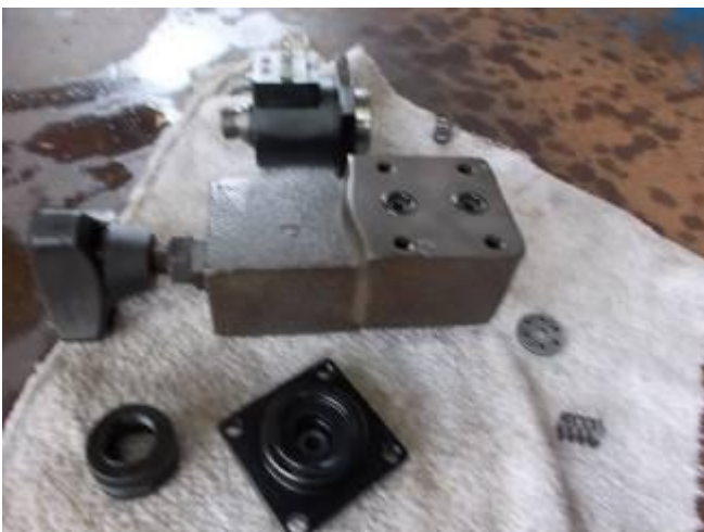
P32: The pressure controller was in the purification. It was then a slide in the hydraulic block jammed.
