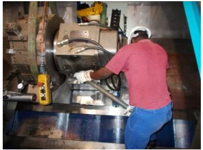
P15: The turret of the Mega Bore was inclined to 100 mm travel 1 mm. So again a big crash.
