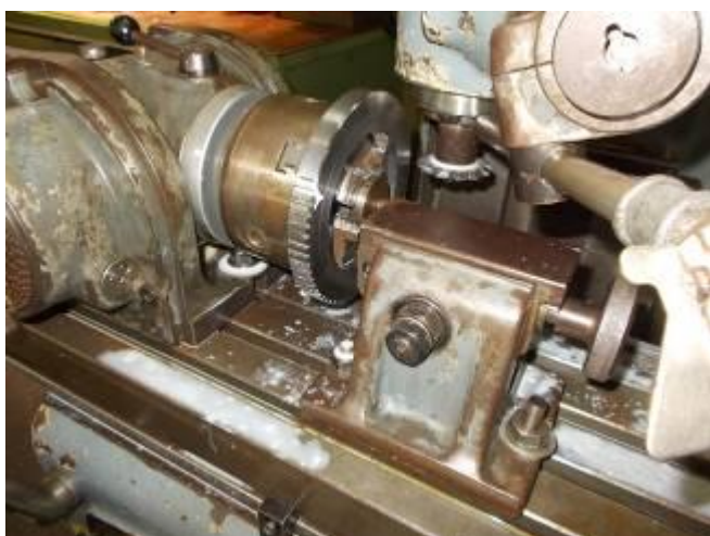
P38: the large gear is re-established. Unfortunately, with the module 2.5 mills, instead of the 2 module cutters. Here we have to gear training with the machine people. They do
