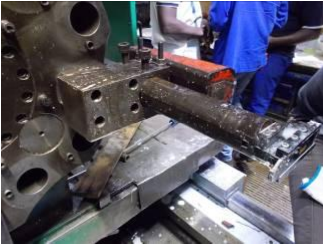
P70: to make a Innedrehstuhl of an outer turning tool, was complicated because the geometry had to be adapted. In other words, an outer steel has a different clearance angle than an inner steel.
