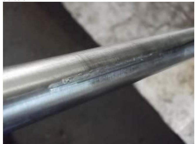
P4. A shaft on which the shift fork runs, has eroded. Unfortunately, the material pairing steel on steel was chosen. It gives only a friction of 0.01 with n oil. But there are no lubrication holes. So there is a risk to eat. If brass or PTFE bushing in there, it would also not dry can chew.
