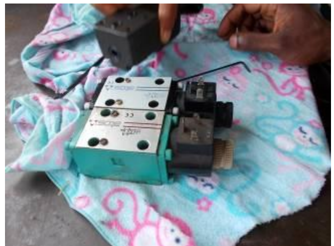
P29: The machine does not move. The valve was replaced. That was not the problem.
