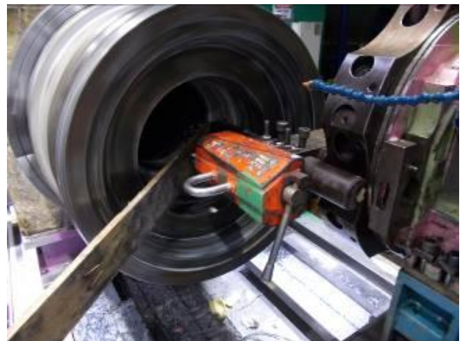
P: Unfortunately, too few steels are available in order to turn vibration free can. It had to improvise something.
