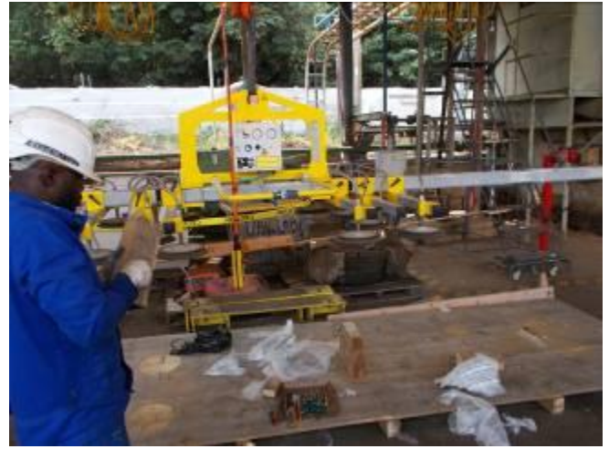
P59: He should lift plates up to 50 mm thickness and 2600 x 1300 mm
