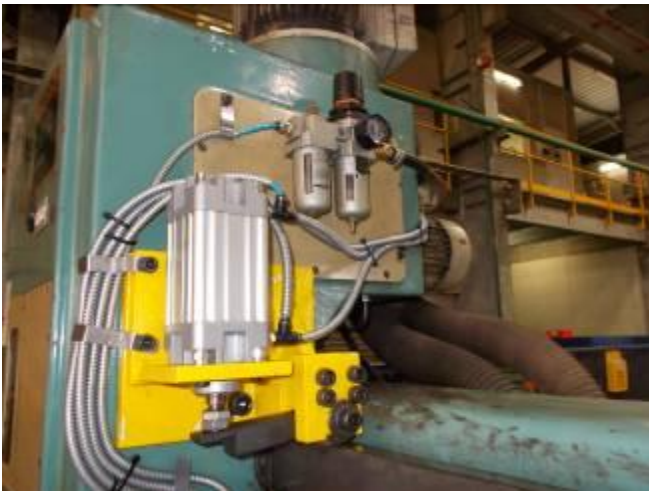
X54: The lines were protected against chips. Such protection hose, we also need to take in the order list. We still had a few feet in the camp.
