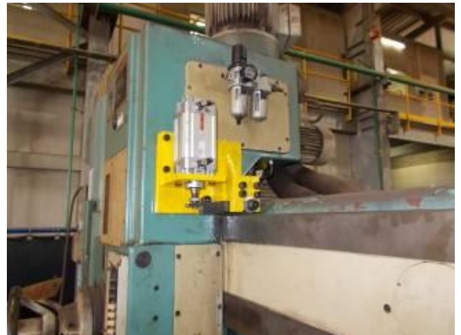
P51: At this drill is a brake outside in cultivation. The original brake is inside. Several times a disassembly was required. Since everything had to be dismantled. Always stop for about 3 days. Now peace will be.
