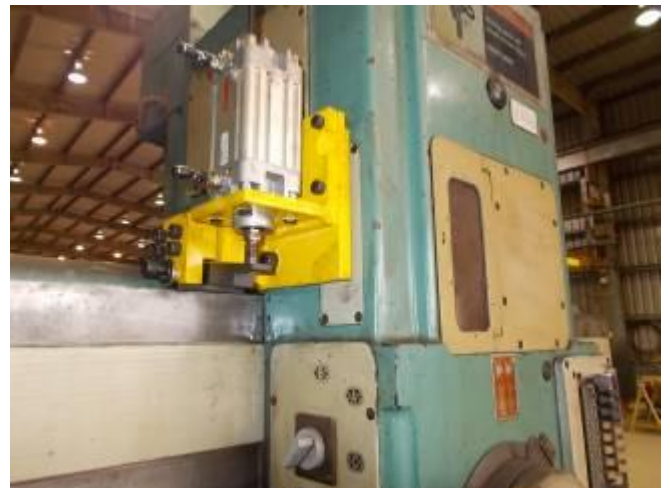
P52: The brake clamped via a lever with 1,200 kp x2.
