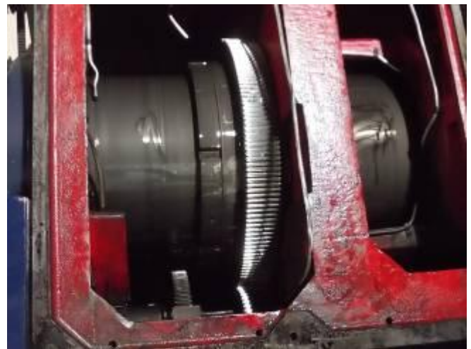
P3. Everything inside is studded with a dark lining. It is an abrasion.
