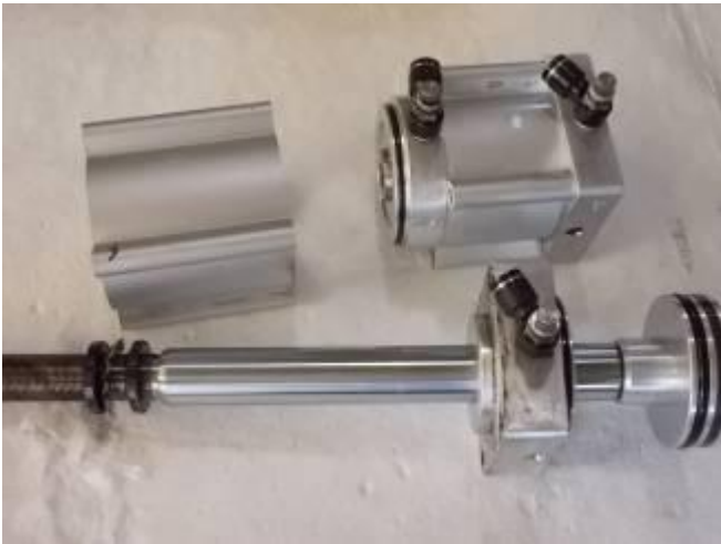
P6: The two cylinders that move the shift forks
