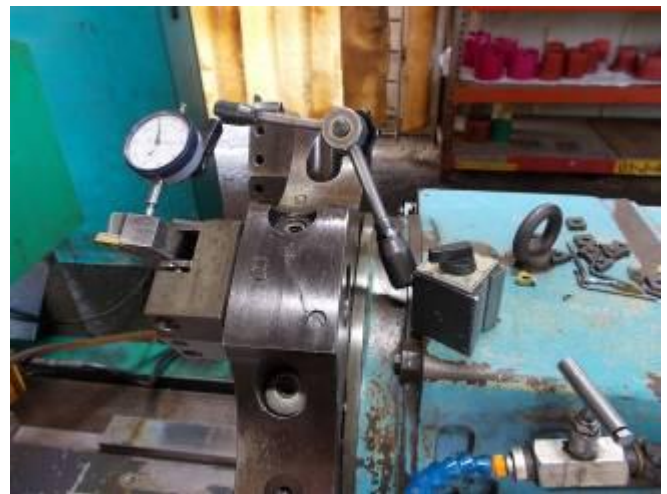
P26: The turret must be without play, otherwise it will vibrate during rotation. This means that the quality requirements are not met.
