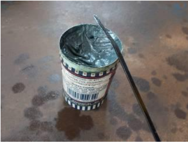
P30: With lapping paste the clamping slide has yet been made accessible. This has to be cleaned very well again. Not the residue then lapping.
