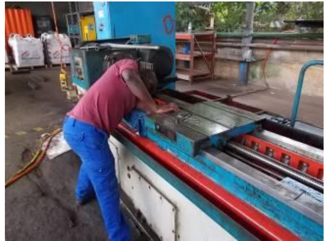
P60: The deep hole drilling machine "TBT TIBO" lost per day several liters of hydraulic oil in the working oil. It had to be dismantled 2 sled. Doing some maintenance work could also be made equal.
