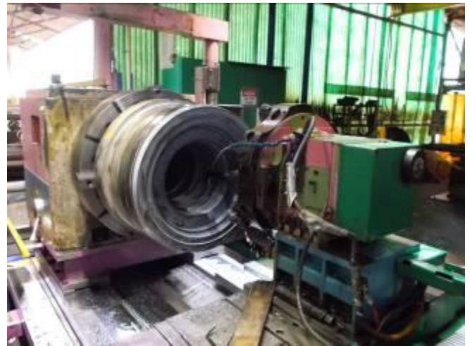
P69: The workpiece on the Gornati is difficult. Fortunately the machine bed is wide and stable. The feed force good enough.
