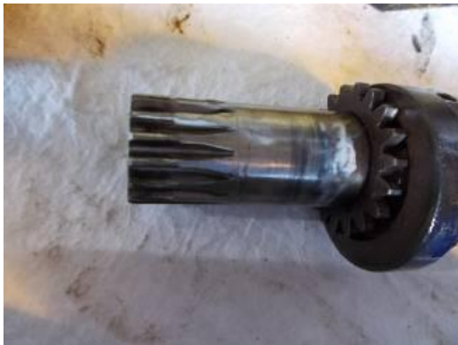
P36: The defective wheel in the feed gear
