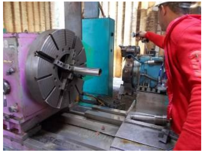
P25: The conicity of the workpiece the headstock is calculated. 7 pages protocol for VAM. 14 pages has the internal protocol.
